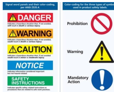
Gambar 1. Standar ANSI Z535 Safety Signs and Labels
